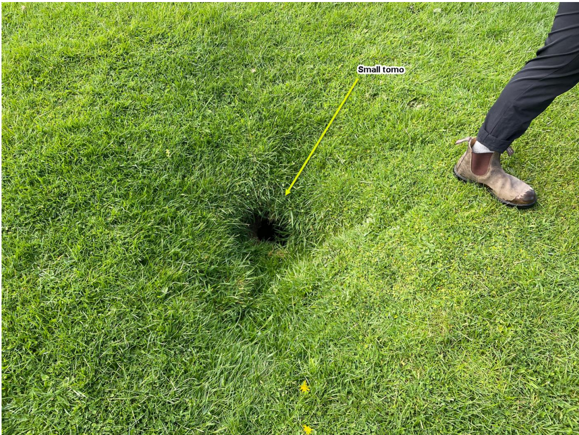
Figure B.4B Example of small tomo found scattered within the catchment areas of both bunds
